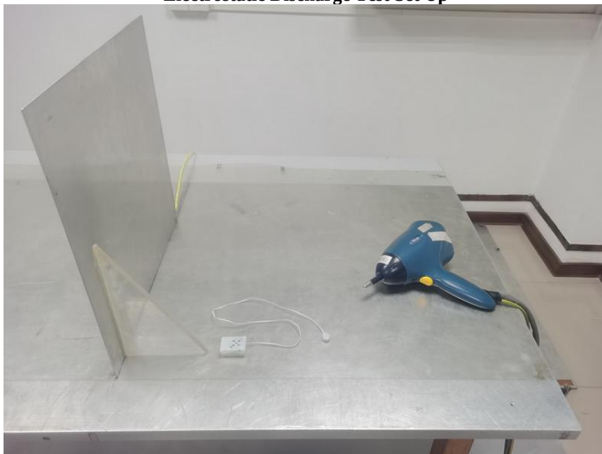
Electrostatic Discharge Test Set Up
