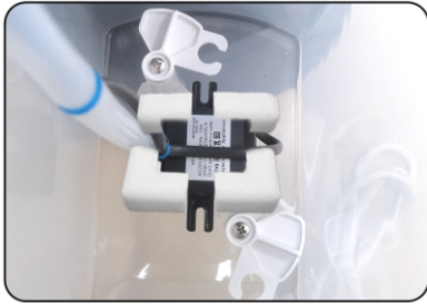
1. Remove the foam around the pump
