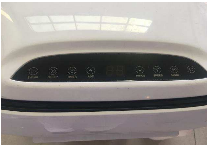
Photo 3 - control panel view of OL-KYR35-A5B
