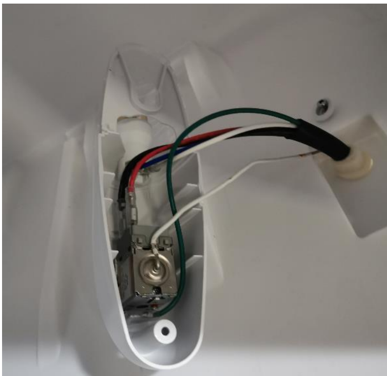
Photo 14 - General view of thermostat box for representative models BC-132BNL, BC-132CNL and BCD-95ANL with LED lamp
