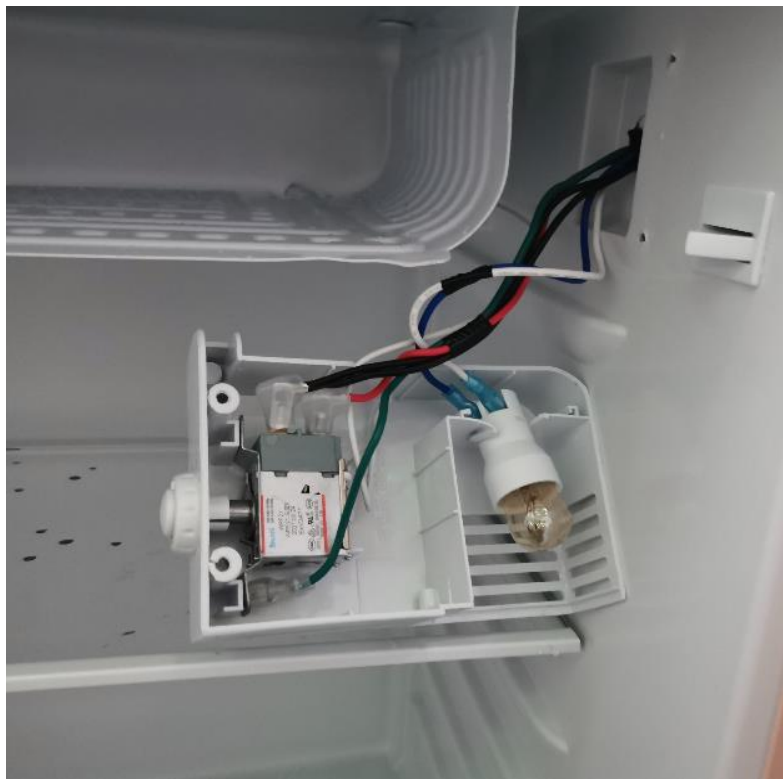
Photo 4 - Detail view of thermostat box for models BC-132AN Series without wire connector
