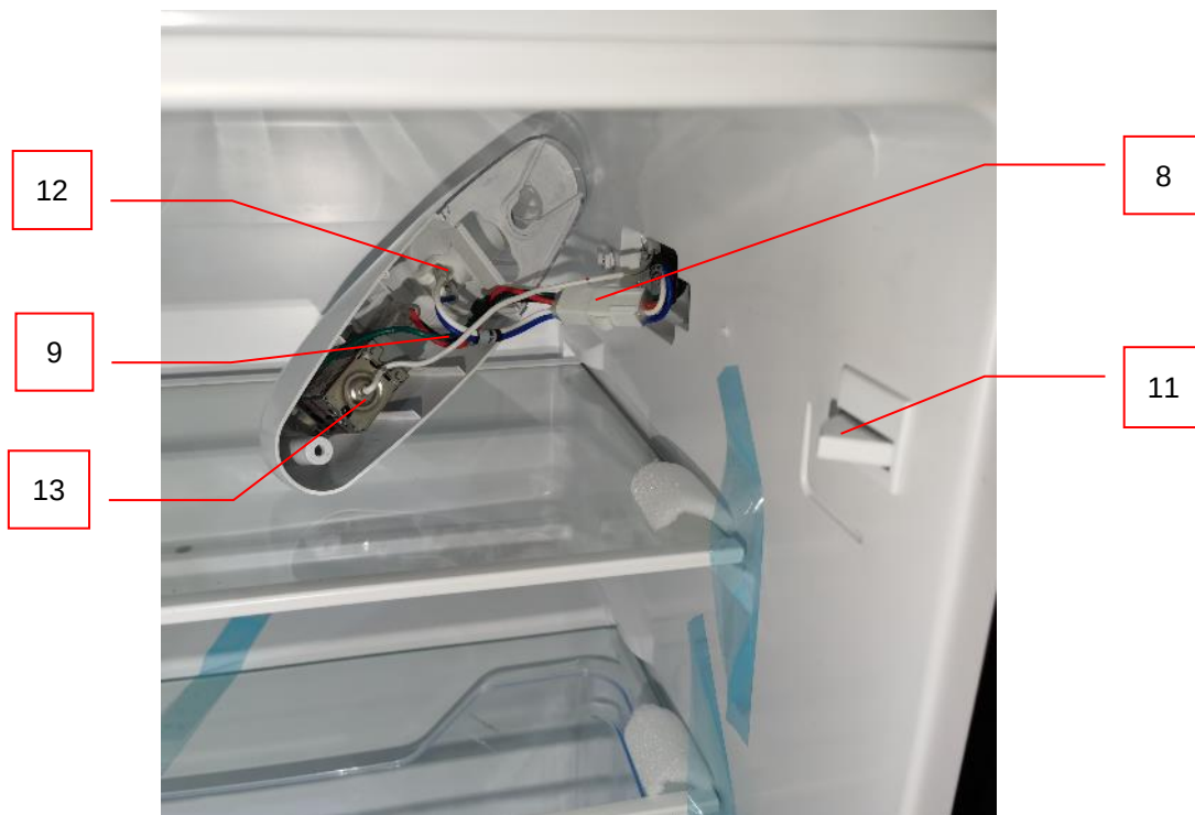
Photo 12 - Interior view of thermostat box for model BCD-95ANB
