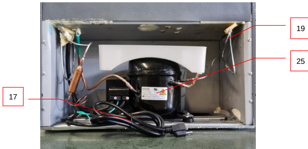
Photo 42 - Detail view of compressor compartment for model BC-428AN
