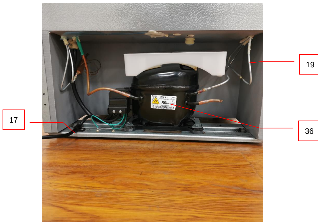
Photo 46 - Alternative compressor FZ50F1G-U for model BCD-138AN Series
