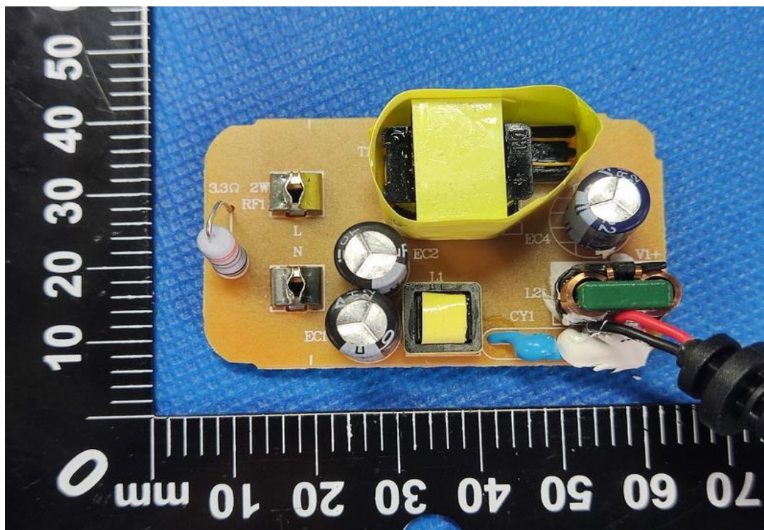
Photo 13 - PCB view with L2, for PCB layout PCB-T984 (Line choke L1: 0501-0027)
