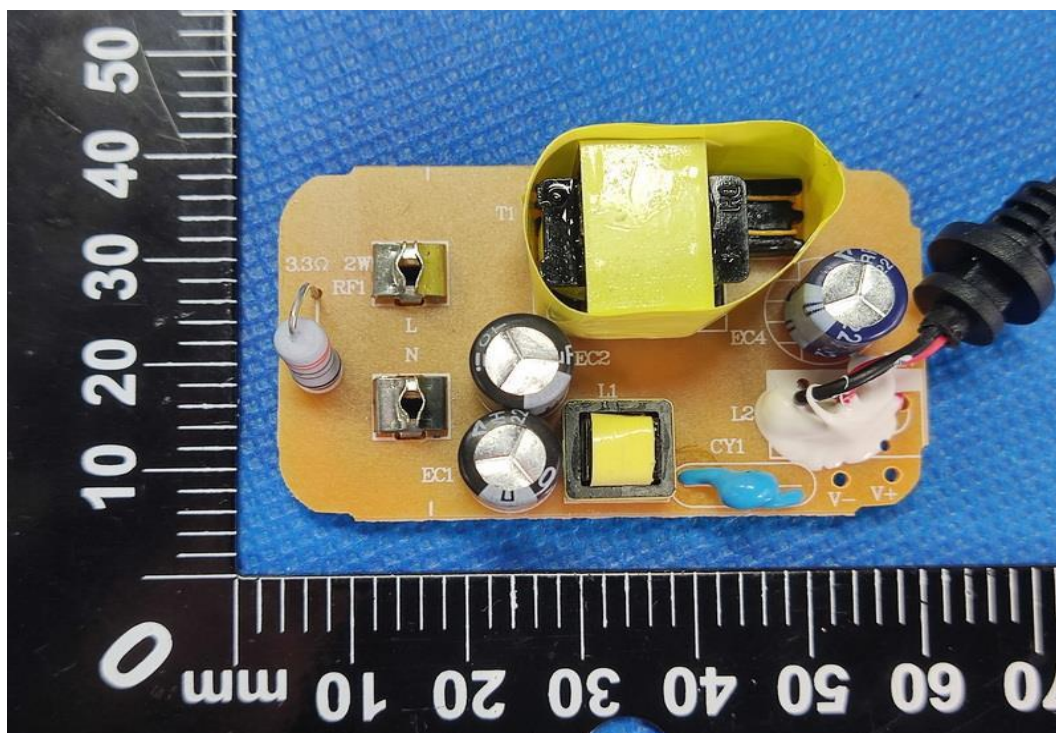
Photo 12 - PCB view without L2, for PCB layout PCB-T984 (Line choke L1: 0501-0027)
