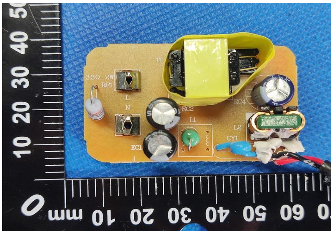
Photo 11 - PCB view with L2, for PCB layout PCB-T984 (Line choke L1: 0510-102K)
