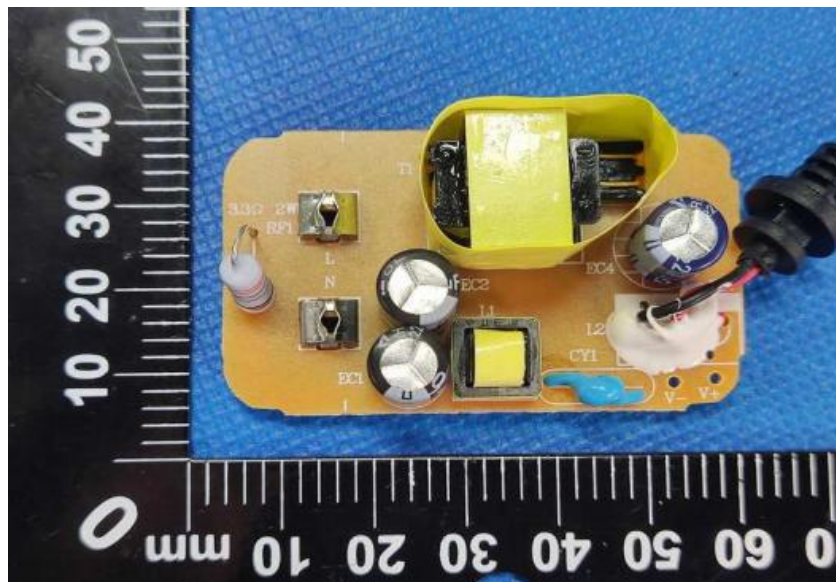
PCB view without L2, for PCB layout PCB-T984 (Line choke L1: 0501-0027)
