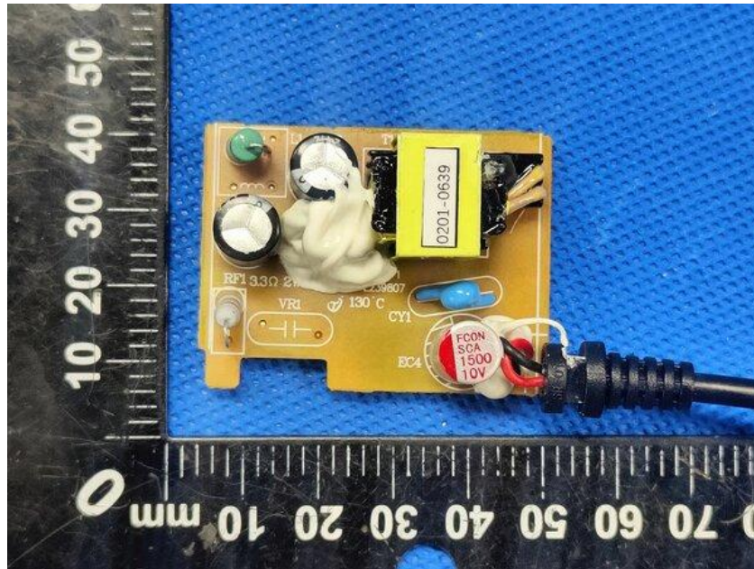
PCB view for layout PCB-T1009-B with transformer 0201-0639
