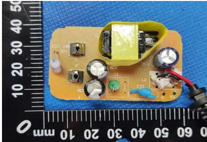
PCB view with L2, for PCB layout PCB-T984 (Line choke L1: 0510-102K)
