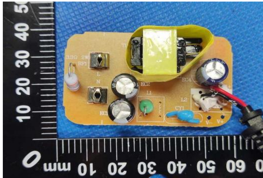
PCB view without L2, for PCB layout PCB-T984 (Line choke L1: 0510-102K)
