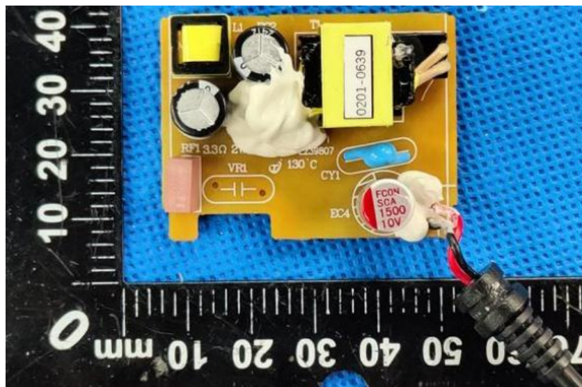
Alternative PCB view for layout PCB-T1009-B with current fuse
