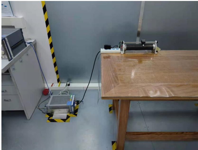
Conducted Emission at The Mains Terminals Test
