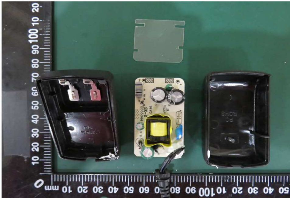
Photo no. 34 - Top PCB view of the Class 2 Power Supply, model RSS1002-*****-W2-D*
