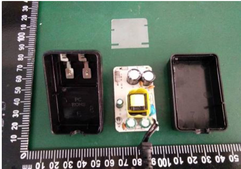
Photo no. 4 - Top PCB view of the Class 2 Power Supply, model RSS1002-*****-W2-E*
