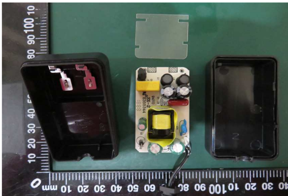
Photo no. 44 - Top PCB view of the Class 2 Power Supply, model RSS1002-*****-W2-E-P*
