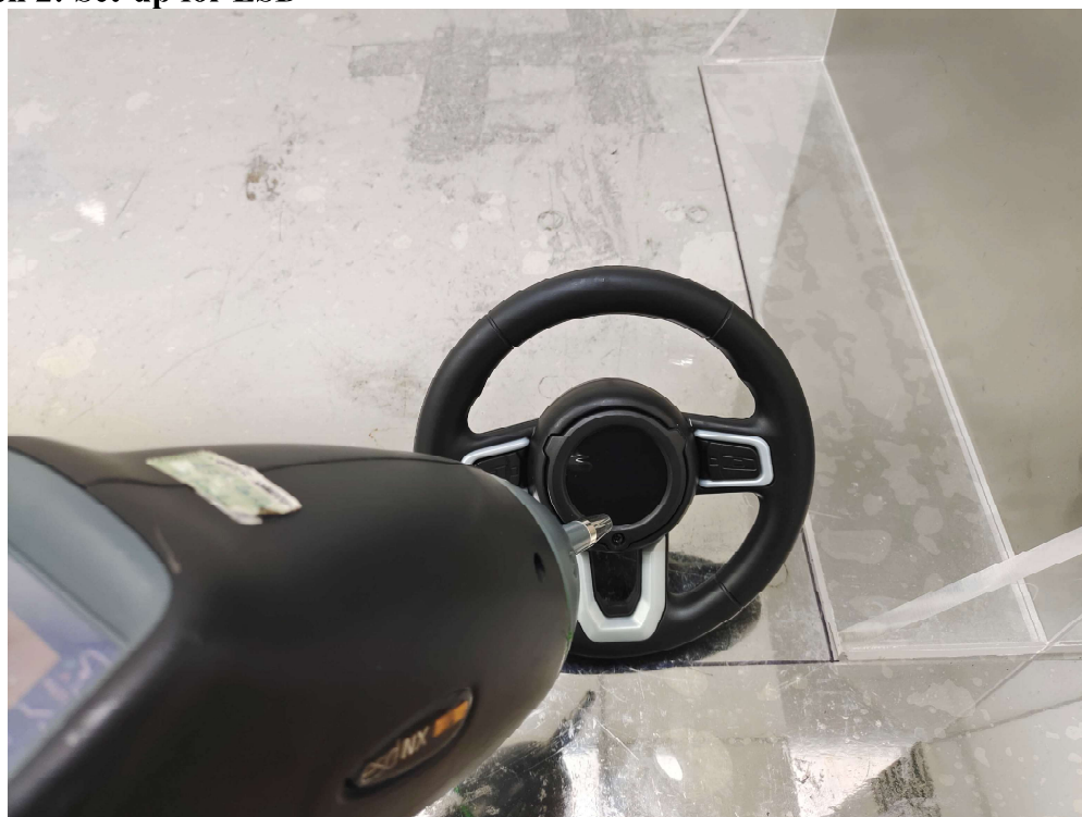
Photograph 2: Set-up for ESD
