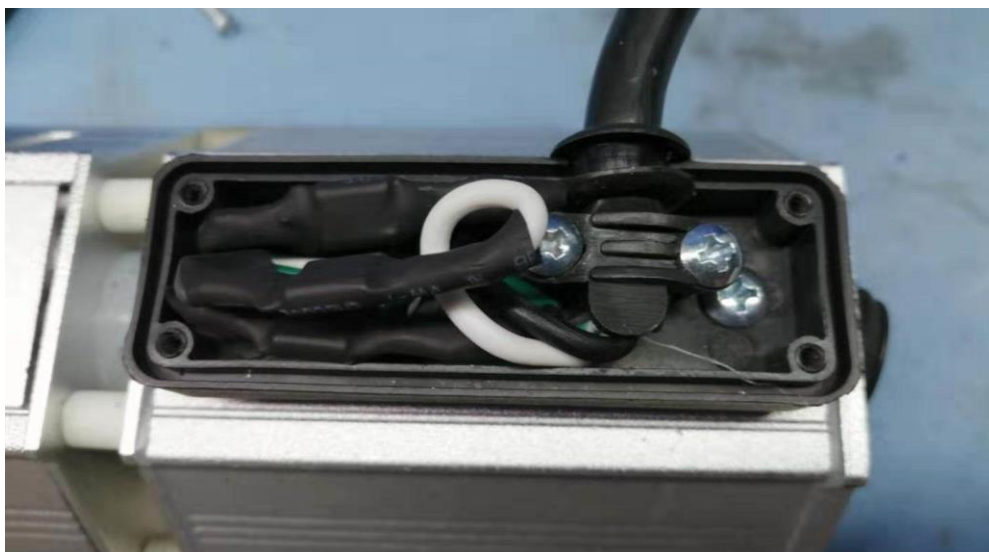
Photo 7 - Internal view of connection box
