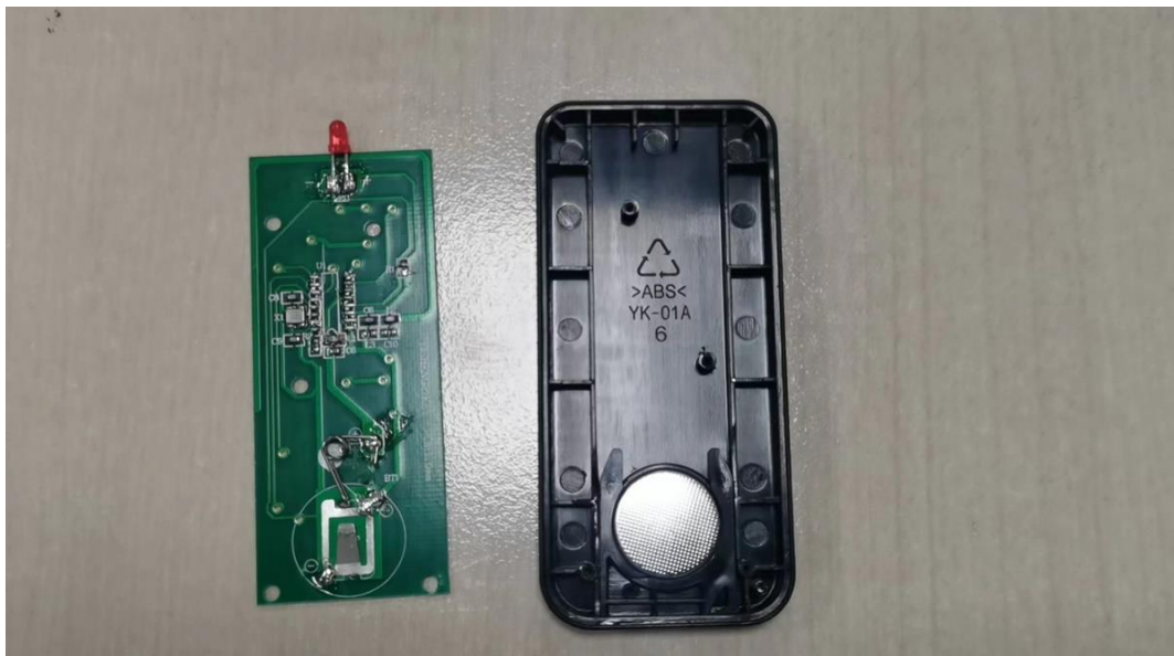
Photo 38 - Internal view of remote controller
